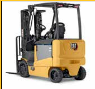
Rear Visibility Low-profile counterweight provides excellent visibility when traveling in reverse.
