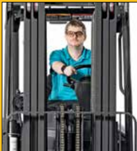
Forward Visibility Narrow mast channels and open overhead guard design for excellent visibility.
