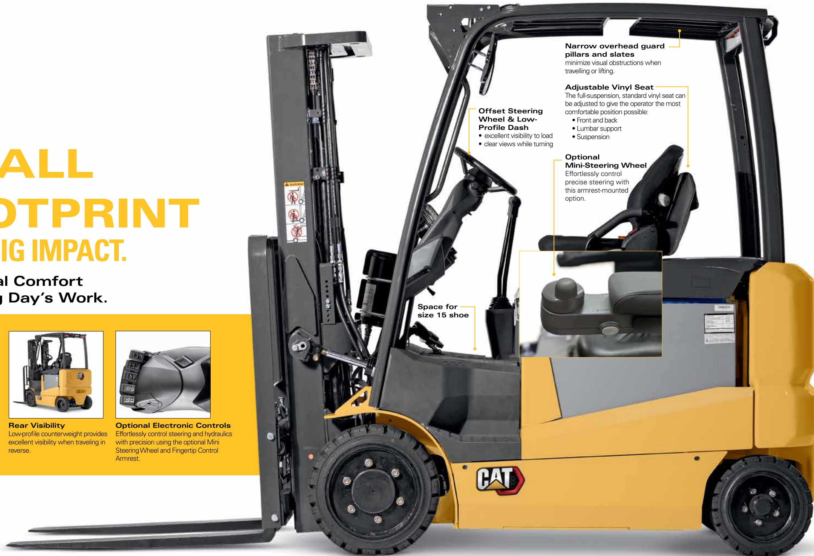
Forward Visibility Narrow mast channels and open overhead guard design for excellent visibility.
